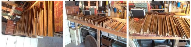
There were a total of eight panels, one of which included the access for the electrical outlet. The aesthetics of the piece meant that the width of the boards that comprised each panel had to be somewhat random. Hence, you must cut boards with varying lengths and widths, lay them out, and organized them *before* you start gluing anything together.
