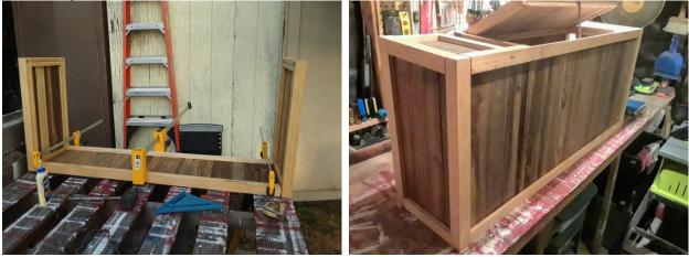
The sub-steps of this step had to be done in order. The end panels had to be completed first because they would ultimately become the ends for almost every other panel. Likewise, the front panel had to be in place before the top because the top uses the front as one of its ends. In the photo on the left you can see the end panels finished and in place while the bottom is clamped while the glue dries.
